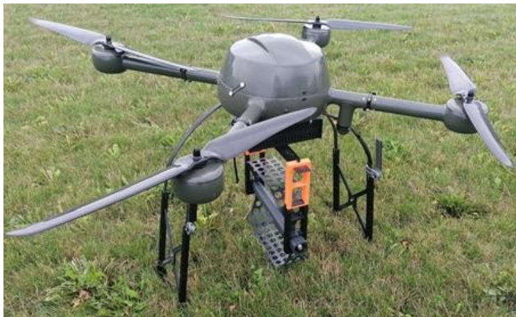
Figure 4 – Example of a drone prepared for a frequency spectrum measurement system.
