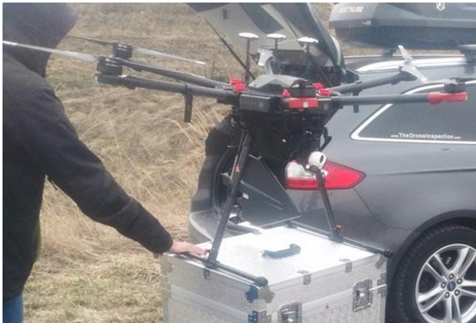
Figure 3 – Example of a drone equipped with a frequency spectrum measurement system.
